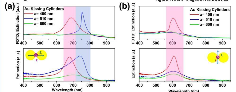
Figure 8: Theoretical and Experimental extinction spectra as a function of wavelength of array of Au kissing cylinders under (a) Longitudinal and (b) Transverse polarizations.
