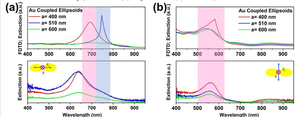
Figure 9: Theoretical and Experimental extinction spectra as a function of wavelength of array of Au coupled ellipsoids under (a) Longitudinal and (b) Transverse polarizations.
