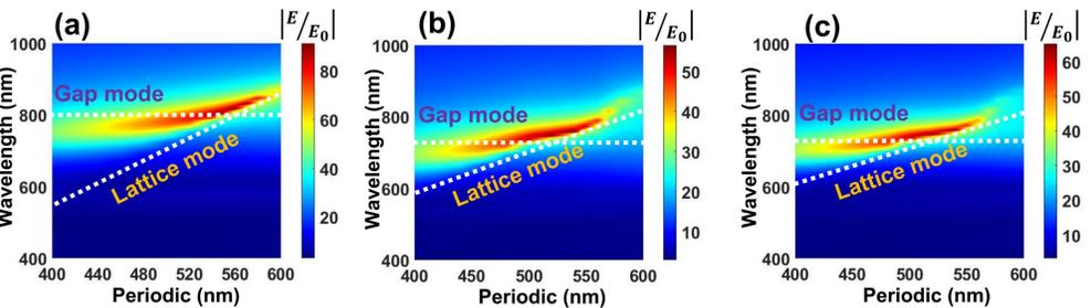
Figure 3: Normalized Electric Field Enhancements of (a) Bowties, (b) Kissing Cylinders and (c) Coupled Ellipsoids Nanoantennas as a function of the wavelength and the period under longitudinal polarization.
