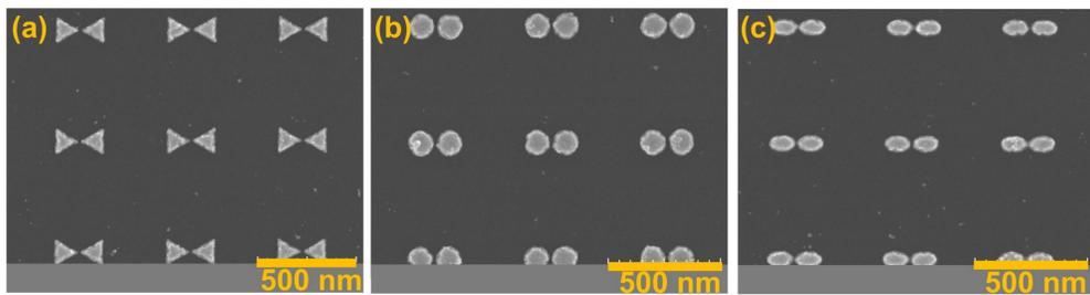
Figure 2: SEM Images of (a) Bowties, (b) Kissing Cylinders and (c) Coupled Ellipsoids nanostructures.
