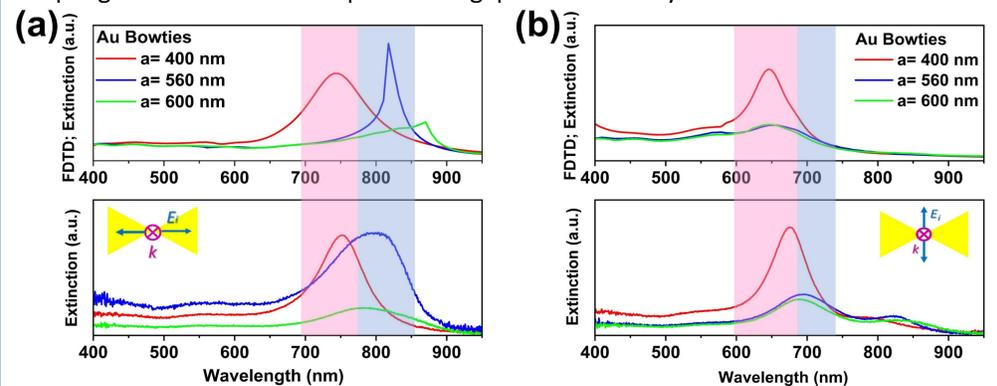
Figure 6: Theoretical and Experimental extinction spectra as a function of wavelength of array of Au bowties under (a) Longitudinal and (b) Transverse polarizations.
