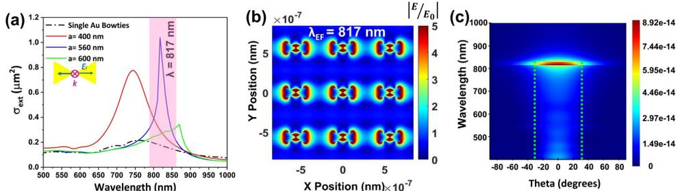
Figure 5: (a) Extinction cross section of arrays of Au bowties, (b) Normalized electric field enhancement which is a direct consequence of the coupling between surface lattice mode and the plasmonic gap mode; and (c) Far-Field projection as a function of wavelength and angle for array of Au bowties (a=560 nm). The far field is confined within a 25° cone of collection with a maximum intensity at the center of the cone.
