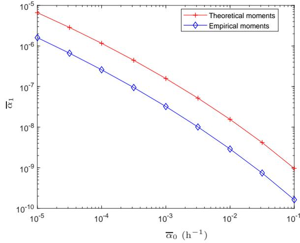
Figure 4: The probability  $\bar{\alpha}_1$  as a function of  $\bar{\alpha}_0$  for SNR  $-30$  dB calculated by using theoretical moments (26), (27) and empirical moments obtained by a  $2 \cdot 10^3$  Monte-Carlo simulation.
