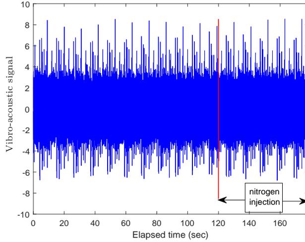
Figure 6: The mixture of the IKHAR and DIADEMO records following (30) – (31). The leak of the HE is simulated by the nitrogen injection at 36 bar pressure starting from  $t_0 = 120$  sec. The SNR is  $-23$  dB.
