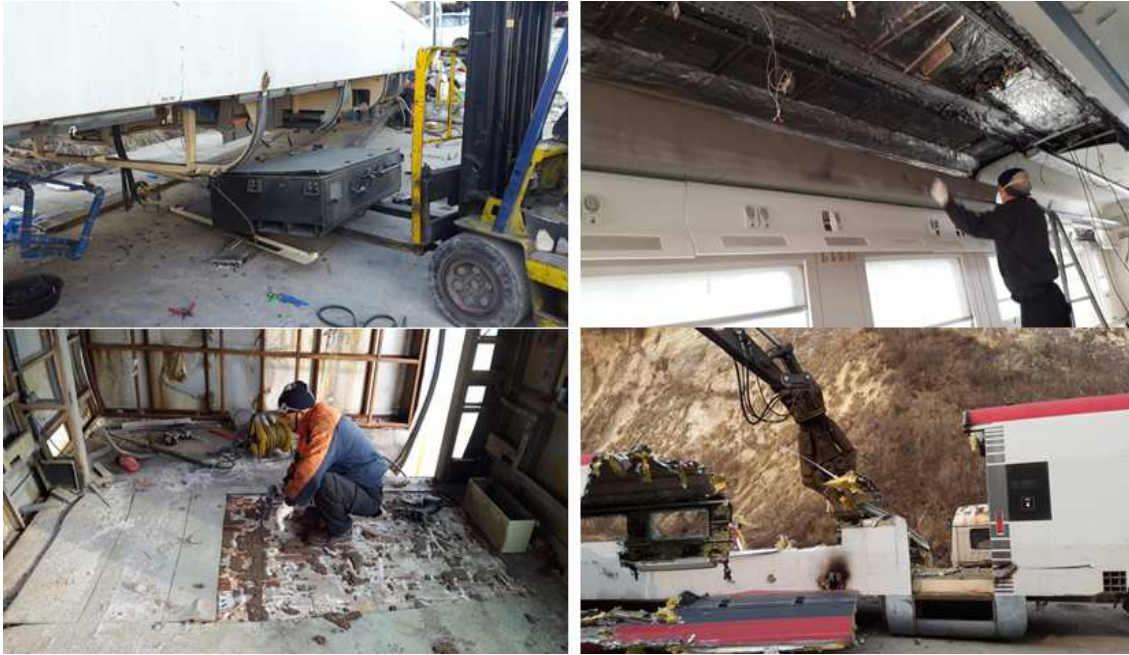
Pretreatment and dismantling steps of End of Life Rolling Stock (ELRS)
