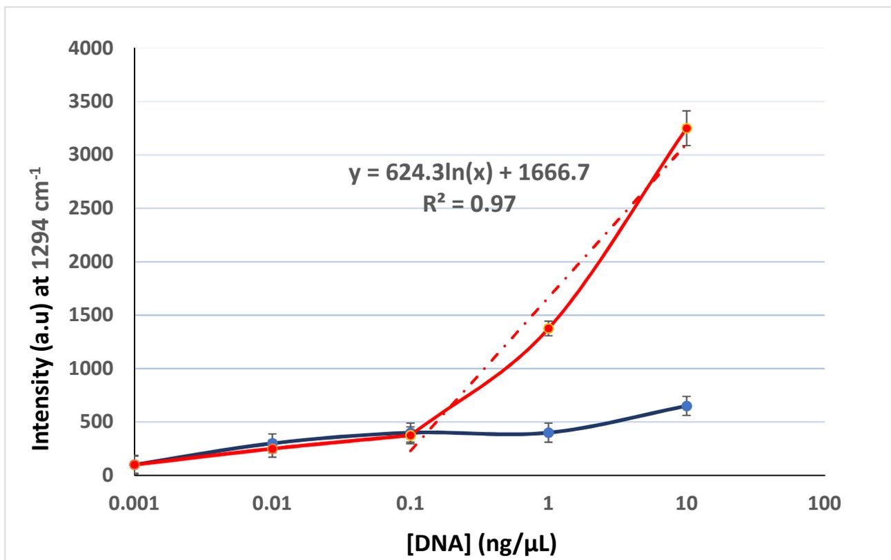
**Fig. 5.** Calibration curves of specific and control *Brett*-genosensors based on SERS measurements.
