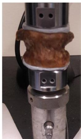
Figure 2b: Lumbar vertebra after failure. Localization of the fracture at the middle of the vertebral body.
