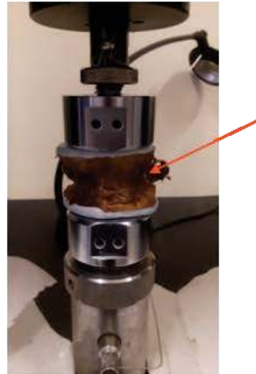
Fig. 5. Lumbar vertebra after failure. Localization of the fracture in the middle of the vertebral body
