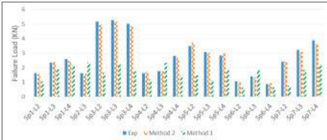
Fig. 7a. Experimental and computed failure loads for the nineteen vertebrae (Method 1 and Method 2)
